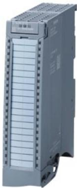
SIMATIC S7-1500, digital input module DI 16x24 V DC AUX; 16 channels in groups of 8; for 24 V encoder; sensor supply 24 V DC; input type 2 (IEC 61131); input delay parameterizable 0.05..20 ms; isochronous mode up to 250 µs; integrated counting function up to 20 kHz; pulse stretching; chatter monitoring; signal inversion diagnostics; hardware interrupts: front connector (screw terminals or push-in) and, if applicable, order shield set separately
