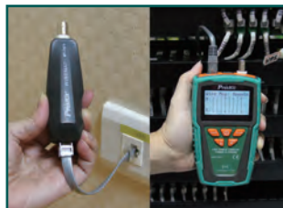
Verify LAN/ Telephone / Coaxial cable condition
