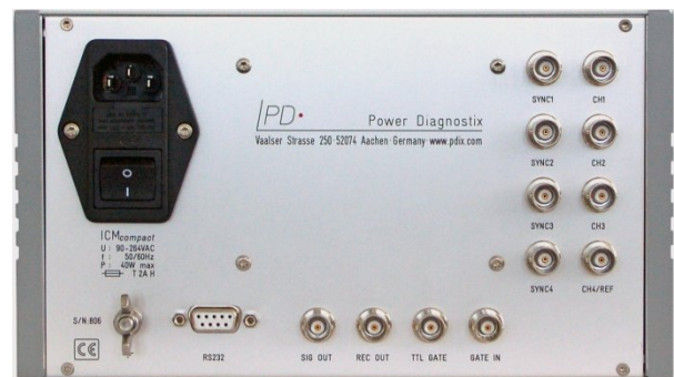
Back of ICMcompact with MUX4 option, RS232, and RIV measurement
